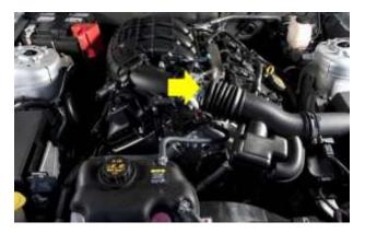
5. Remove the lid that covers the air filter and the hoses that connect to the intake tube. This section of air intake should now be able to be placed to the side.
