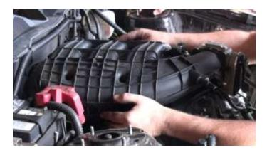
15. Tighten the 7 bolts until snug to ensure a perfect seal. Place close attention not to over tighten. The included spacer takes up some of the thread depth of the factory bolts but still has plenty of threads to ensure a proper fitment.
