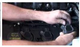
10. Your new Granatelli coils include a specifically designed spacer that allows for the higher capacity coils to work properly. Therefore, it requires one each (per coil) the supplied metal spacer and longer bolt.
