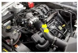
6. Remove the wiring harness that connections to existing throttle body.
