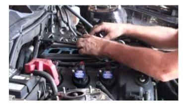
14. Put the upper plenum back in place with the existing hardware still in the manifold holes.
