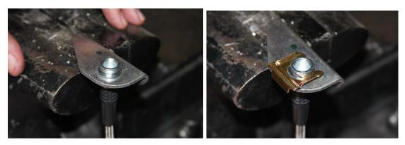
Shown above, This is how easy it is to modify your brackets. The picture to the right shows the retaining clip installed. This is for reference only. It is not recommended that this clip be installed until after the lines are mated.
