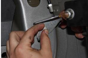
Remove the bolt holding the brake line bracket using a 10mm wrench or socket
