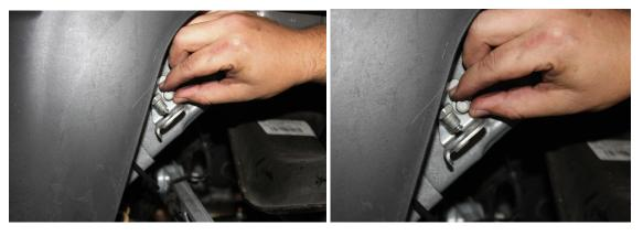
Pictures above represent a view of the rear brackets – The same applies. Drill D shape into a perfect circle
