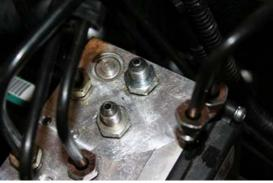
7. Using a 13mm wrench loosen the 2 ABS lines shown in the picture above and install the proper male to male adapters. (2) 280070. Note – No Teflon tape is used in this step
