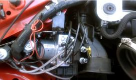
8. Place the two adapters male to male into the ABS unit, followed by the top two lines from the line lock unit.
