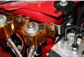
6. Reinstall the factory ABS bracket by reversing the steps above and then fasten the line lock assembly into the two holes you just drilled using 2 of the supplied  $\frac{1}{4}$  x 20 nuts, flat washer and bolts. Here is the line locks installed before the lines are hooked up.
