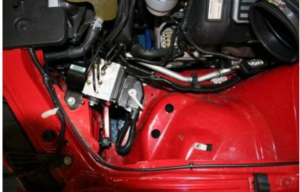
2. Using a 10mm socket or wrench remove the (1) 10mm bolt that fastens the stock air box to the fender on the driver's side. Using a flat blade screwdriver loosen the clamp that connects the soft below tube to the factory or aftermarket air box.
