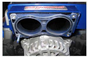
Important: Retain the Factory O-Ring on intake manifold
