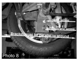
4. Confirm GMS LCA relocation bracket is parallel with the ground. This confirms axle alignment. -Tighten up bolt (see photo 8).
