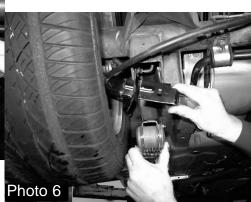
2. Note location on parking brake cable bracket that you need to cut. Cut it off. We used an abrasive cut-off wheel but a hack saw works as well. This bracket needs to be cut to accommodate the new LCA relocation brackets. Note: - You will
