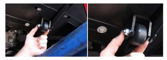
3. Bumper Savers are to be mounted to both insides of the lower radiator support arms so repeat this step on the other side (inside of support on left and right) as well.
